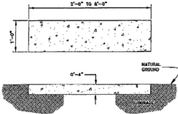
**Figure 1. - Typical section for Concrete Foundation.**
