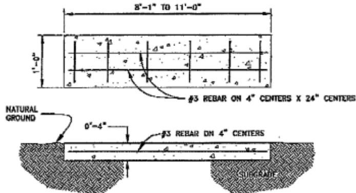
**Figure 2. - Typical section for Reinforced Concrete Foundation.**
